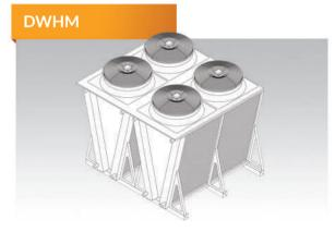
Modular drycooler with multiple heat exchangers which allows to break system into separate independent circuits. Units are based on modular structure frame, which allows to extend unit to large capacities. W shaped large units. Provides large heat capacity within limited area and higher energy class in comparison with flat units. Finned pack heat exchanger with copper tubes and aluminum fins. AC and EC fan motor technology. Powder painted galvanized steel frame.
