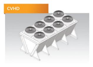
Large capacity range air cooled condenser series for refrigeration applications. Available heat capacity range – over 1 MW upon nominal conditions. V shaped large units. Double heat exchanger and double fan row provides large heat capacity within limited placement area. Finned pack heat exchanger with inner grooved copper tubes and aluminum fins. AC and EC fan motor technology. Powder painted galvanized steel frame.
