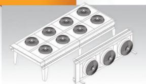
Wide capacity range drycooler series. Flat shaped various size units. Finned pack heat exchanger with tubes and aluminum fins. AC and EC fan motor technology. Powder painted galvanized steel case.
