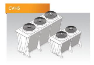
Wide capacity range air cooled condenser series. Available heat capacity range – up to 800 kW upon nominal conditions. V shaped various size units. Double heat exchanger and single fan row provides large heat capacity within limited placement area and higher energy class in comparison with flat units. Finned pack heat exchanger with inner grooved copper tubes and aluminum fins. AC and EC fan motor technology. Powder painted galvanized steel frame.
