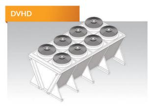
Large capacity range drycooler series. V shaped large units. Double heat exchanger and double fan row provides large heat capacity within limited area. Finned pack heat exchanger with copper tubes and aluminum fins. AC and EC fan motor technology. Powder painted galvanized steel frame.
