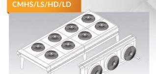
Wide capacity range air cooled condenser series. Available heat capacity – up to 800 kW upon nominal conditions. Flat shaped various size units. Finned pack heat exchanger with inner grooved copper tubes and aluminum fins. AC and EC fan motor technology. Powder painted galvanized steel case.
