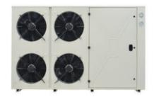
Condensing units for shops usually have one or two compressors installed, depending on the application. For medium temperature it is one rotary (up to 8 kW at -10 °C evaporating temperature) or reciprocating (8-20 kW at -10 °C) compressor, for low temperature – two reciprocating compressors (up to 15 kW at -35 °C). This type of condensing unit is compact and easy to install.
